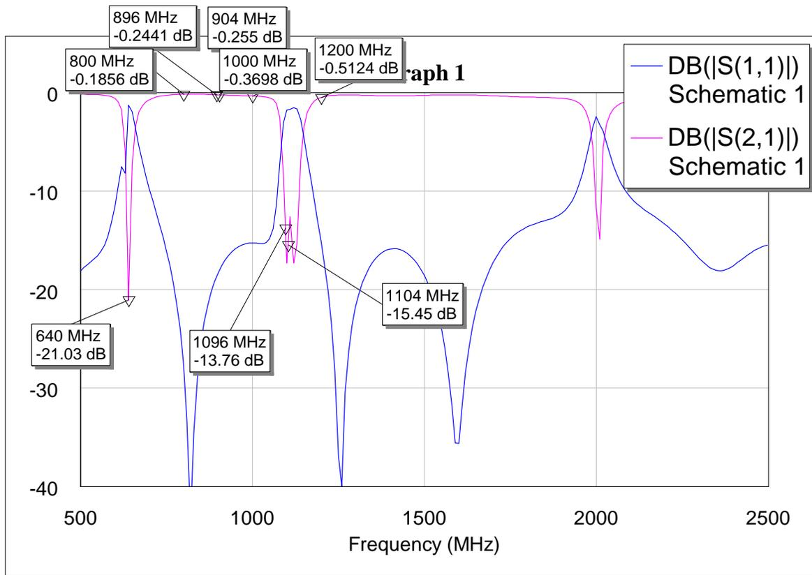
The response meets 10-20 dB attenuation specification in the 1.096 GHz to 1.104 GHz band. 0 points are incurred.
